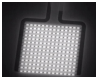
Printed heating as a thermal image
